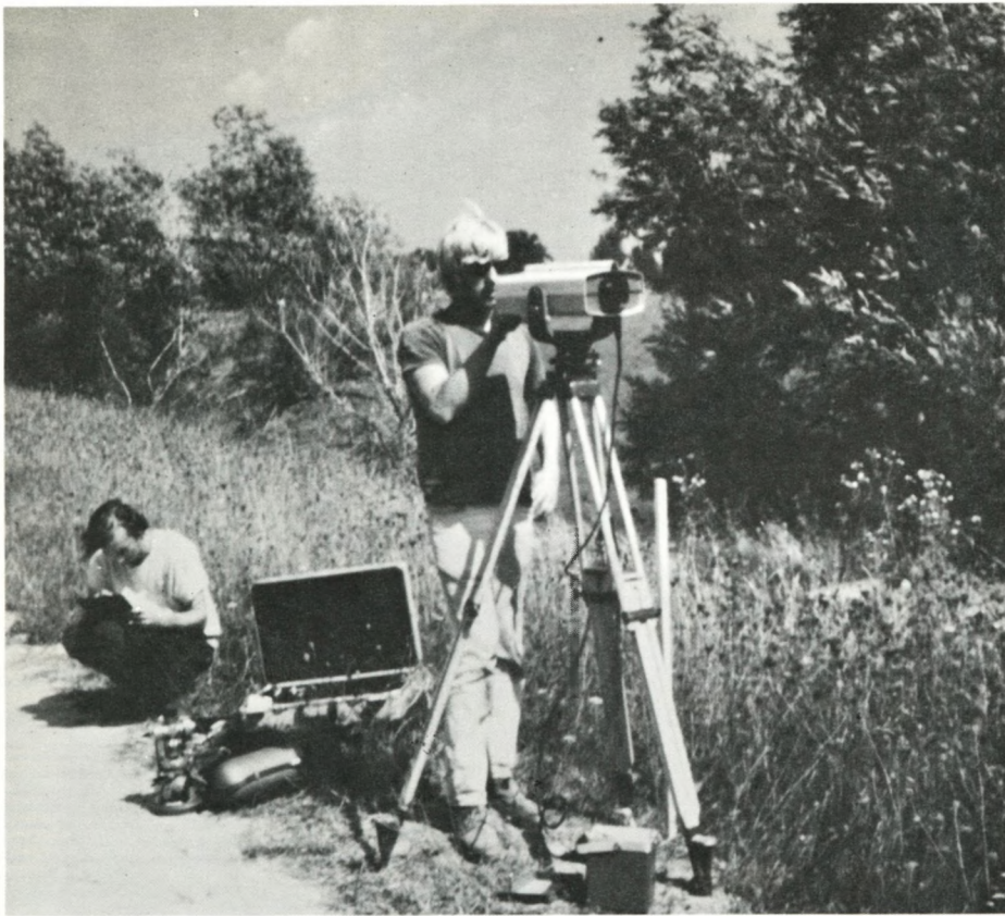
Hewlett-Packard Distance Meter set up on bank of Thames River
