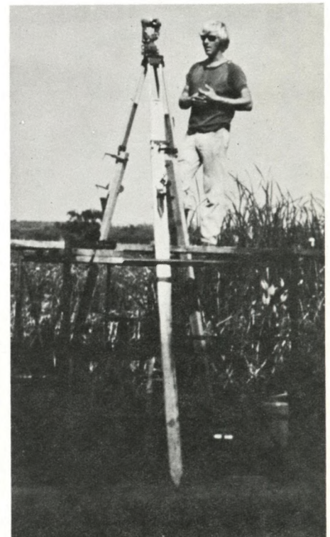
WILD T-2 mounted on 2" x 4" x 8' legs with operator on Safeway scaffolding. Location: Bradley Marsh, Chatham, Ontario.
